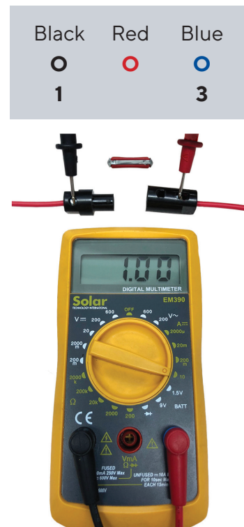
Meter connected to a wire with a reading of 1A
